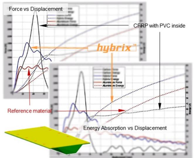
The results from the investigation confirm that the CFRP beam with inside PVC foam absorbed least amount of energy at the impact test and it was only located in the elastic region of the material. This indicates that the structure did not have the ability to plastic deformation which is an important requirement for the proposed application. However, it is possible to reduce the total weight up to 24% lighter than the reference material.
